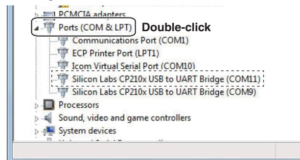
• When the driver is completely installed, "Silicon Labs CP210x USB to UART Bridge (COM\*)" is displayed. The screen shows the USB serial COM port number "11".
